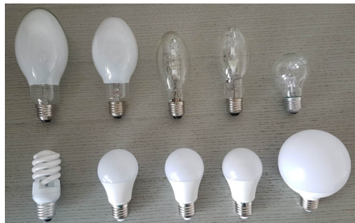
Fig. 2. Light sources used for measurements (from left to right): HG, HPS, MH3, MH4, HAL, CFL, LED6, LED4, LED3, LED0
