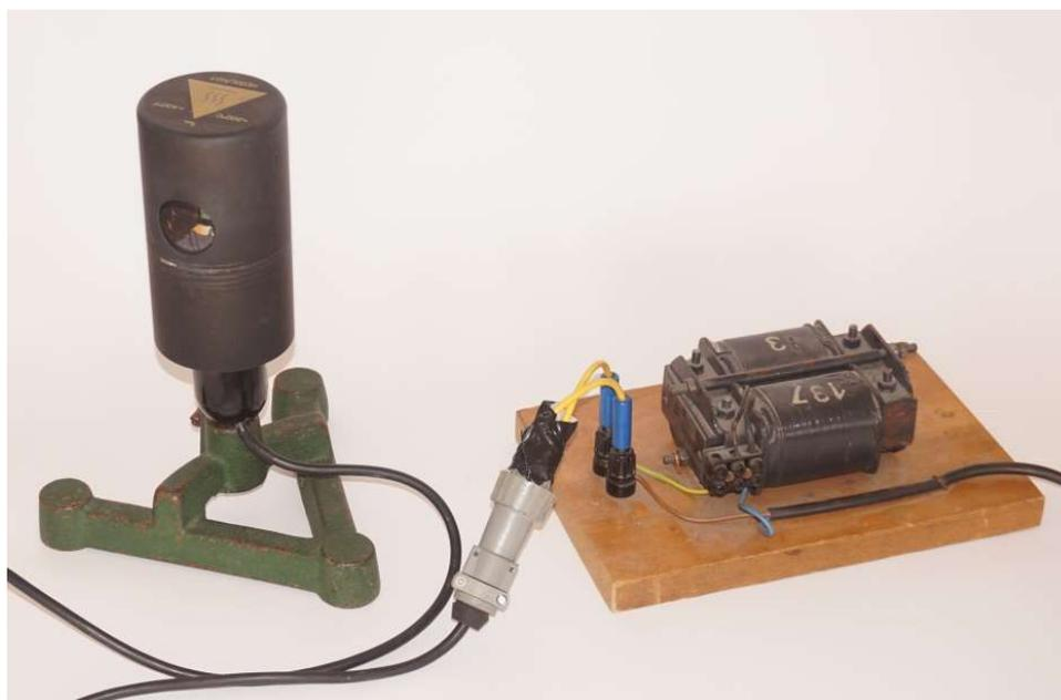
Figure 1 - Leybold 45115 High Pressure Mercury Lamp and in-house matched choke. Luminance  $600 \text{ cd/cm}^2$ , CCT  $\sim 6000 \text{ K}$ , operating current  $\sim 1 \text{ A}$ .
