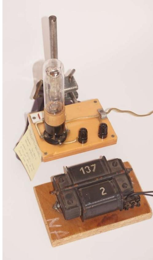
Figure 2 - OSRAM Na/10 Low-pressure sodium spectral lamp with choke and starter.
