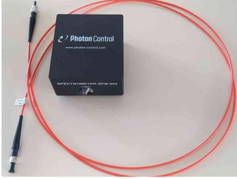
Figure 4: Photograph of the spectrophotometer and the 600  $\mu\text{m}$  core diameter fiber cable.
